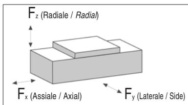
*The capacity of **EL.MORE ELM** series linear units depends on the linear motion system used and may vary according to the loading direction: radial and side.*
