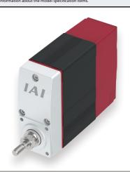
(1) Since the feed screw has no rotation stopper, add a rotation stop mechanism such as a guide to the tip of the feed screw when in use. (If there is no rotation stopper, the feed screw will rotate instead of traveling back and forth.)
