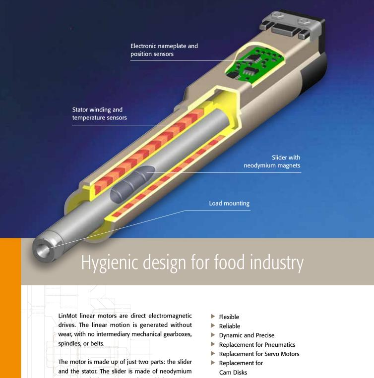
The motor is made up of just two parts: the slider and the stator. The slider is made of neodymium magnets, which are mounted in a high-precision stainless steel tube. The stator contains the motor windings, slider bearings, position sensors, temperature monitoring, and microprocessor circuitry with an integrated electronic nameplate.
