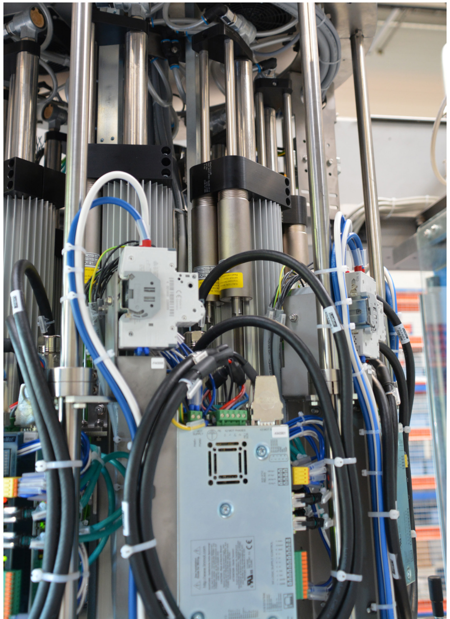
Magnetic springs (in the picture left of the cooling fins) compensate for the weight of the closure spindle and maintain a safe position even when power has been disconnected.
